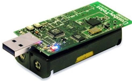
Figure 2.3: TelosB mote open-source platform.
