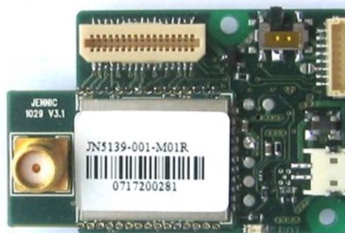
Figure 2.4: iSense modular platform.
